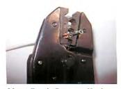
5.Insert Female Connector Heads onto each wire and tighten with crimping pliers.
